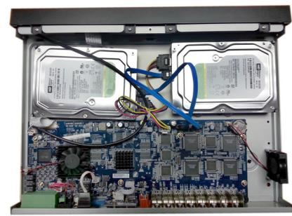
5. Turn over the DVR housing and secure the new HDD to the housing using the four supplied HDD mounting screws.
